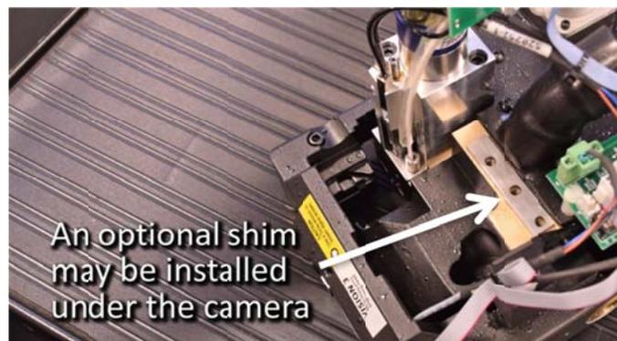
32. Install the camera assembly into the new head.
