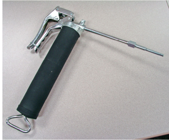
Grease gun with push-on-tube installed
