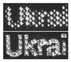
unique algorithm that controls size, shape and placement for unmatched quality. Hybrid Engraving combines the benefits of electro-mechanical engraving and chemical etch, with the unique ability to place cells off the grid. Laser-like quality without the laser expenses!
