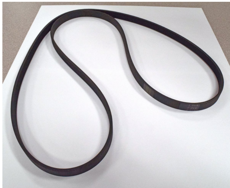
D1120-0055 – Belt, Poly V, 6 Rib, 1562 mm (61.5 inch), Main Drive Belt (Second Generation Spectrums)
