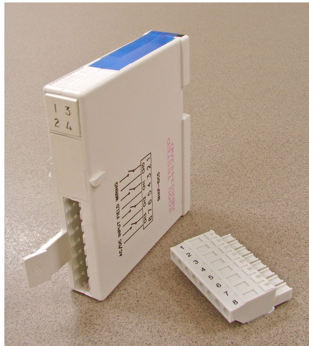
D2580-0064 – Opto-Isolator Module, 4 Channel, Output
