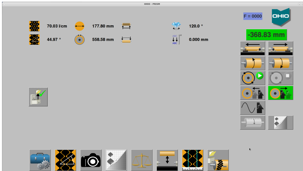
The operator display, or GUI. This is the page seen after start-up, the Engrave page
